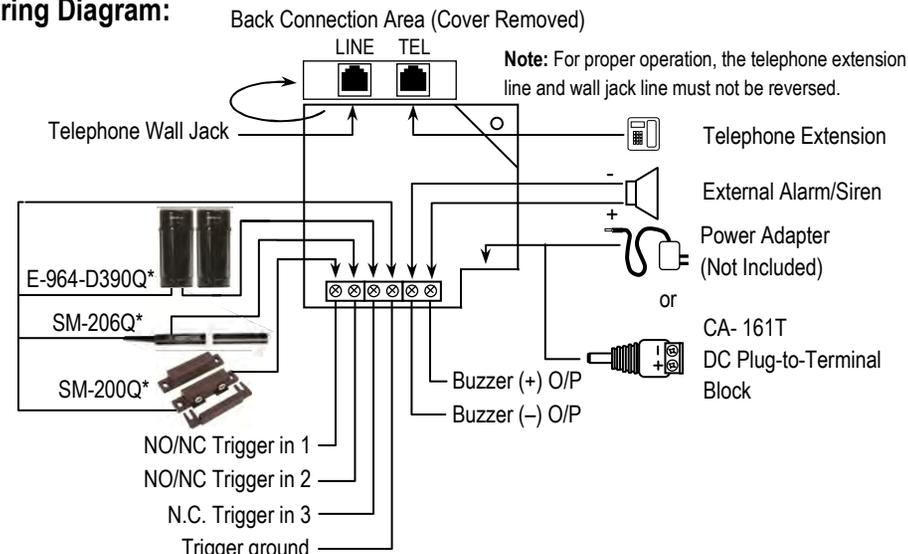
\* E-964-D390Q Photobeam Detectors, SM-200Q Magnetic Sensors, and SM-206Q Concealed Magnetic Sensors shown as examples only: For other sensors and products available from SECO-LARM, please visit our website at [www.seco-larm.com](http://www.seco-larm.com).
