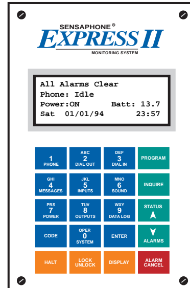
Figure 5-1: Express II Local Display and Keypad
