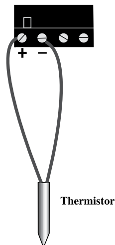
Wiring a Temperature Sensor
